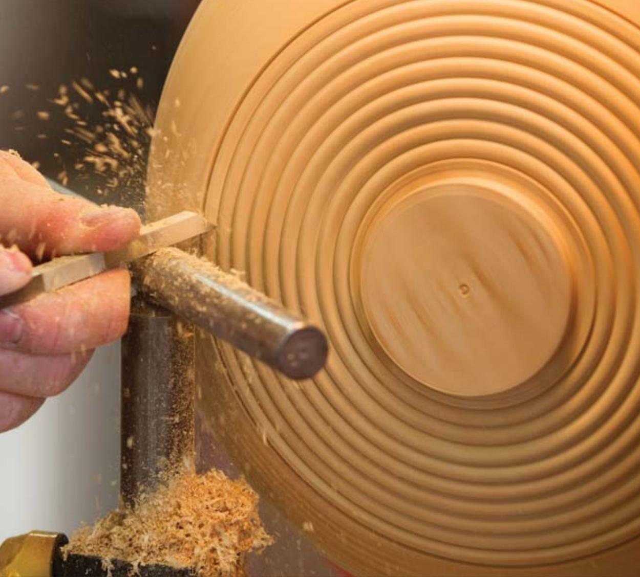
Sue Pritchard carefully directs the sharp carving tool to shape the wood on the lathe. Precision is required to avoid lumps, bumps and chips.
